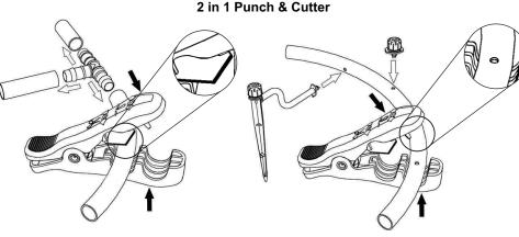
Cuts low density poly pipe and vinyl tubing up to 22 mm OD.
